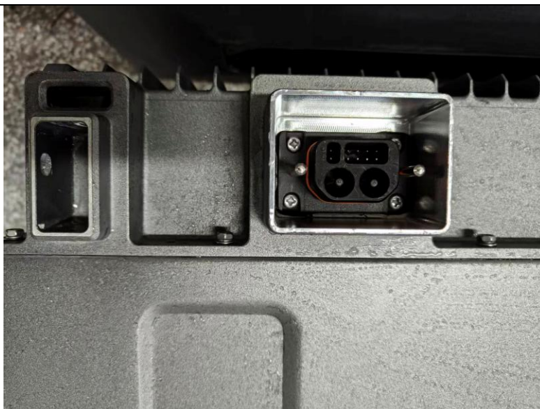
Battery connector of the expansion battery pack (Test without mounting Base)
