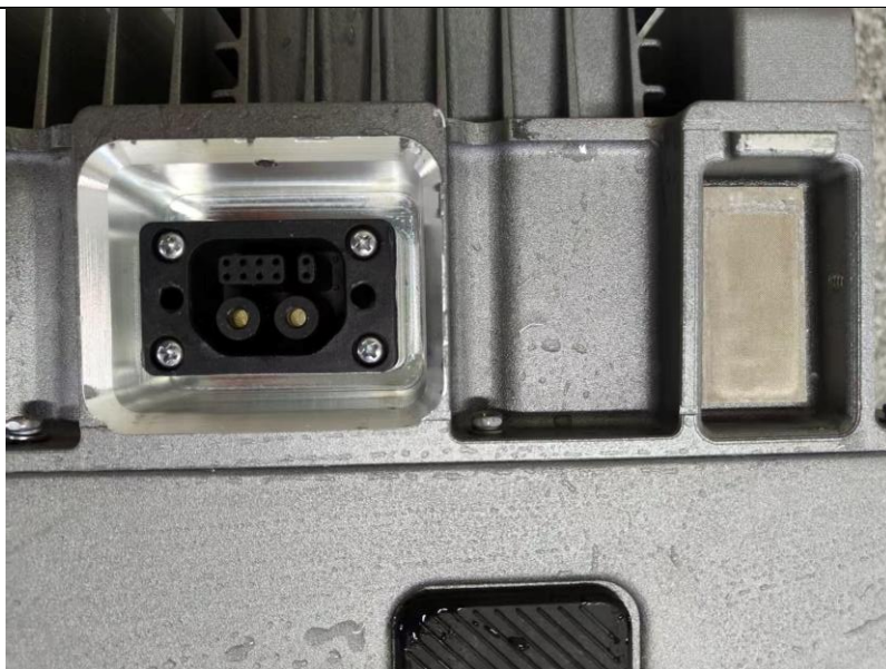
Battery connector of main module (Test without mounting Base)
