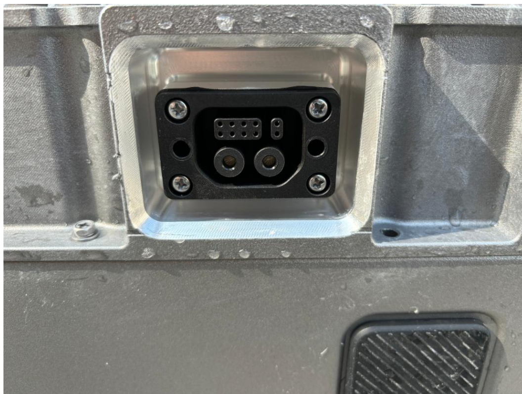
Battery connector of main module
