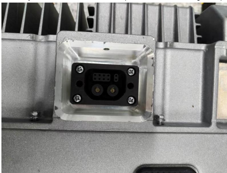
Battery connector of main module (Test with mounting Base)
