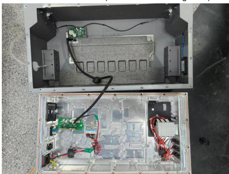
Inside of main module (Test with mounting Base)
