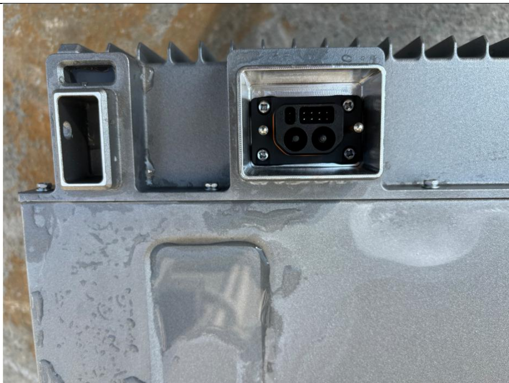
Battery connector of the expansion battery pack
