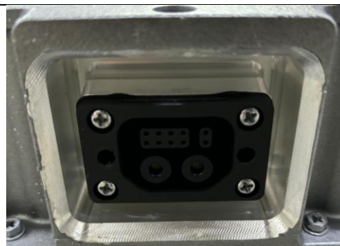
Detail view of Battery connector
